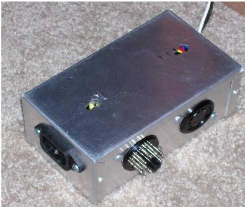
Figure 2: Pictures of the completed adapter. Mounting holes can be seen in the second view - adapter is installed just above the Leslie amplifier.
