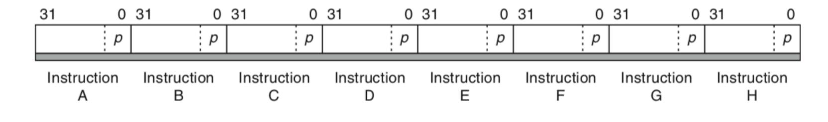
**Figure E.6** Instruction packet of the TMS320C6x family of DSPs. The p bits determine whether an instruction begins a new VLIW word or not. If the p bit of instruction i is 1, then instruction i + 1 is to be executed in parallel with (in the same cycle as) instruction i. If the p bit of instruction i is 0, then instruction i + 1 is executed in the cycle after instruction i. (Courtesy Texas Instruments.)
