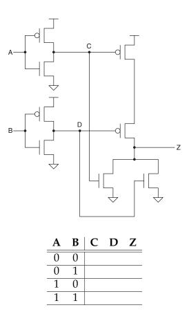
**2.** Referring back to the transistor-level circuit shown in Problem 1, what is **Z** in terms of **A** and **B**?
