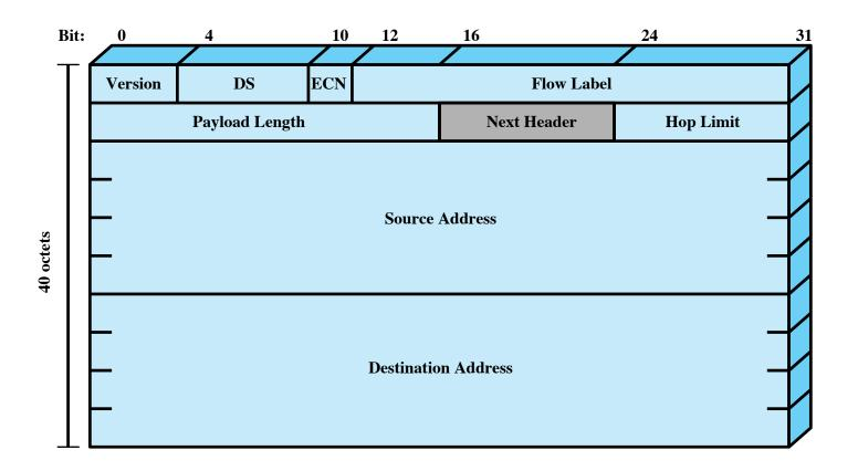
DS = Differentiated services field ECN = Explicit congestion notification field Note: The 8-bit DS/ECN fields were formerly known as the Type of Service field in the IPv4 header and the Traffic Class field in the IPv6 header.
