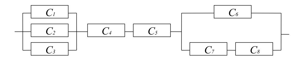
$$S = (C_1 + C_2 + C_3)(C_4C_5)(C_6 + C_7C_8)$$
