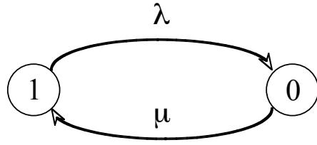
$\lambda$  = failure rate
