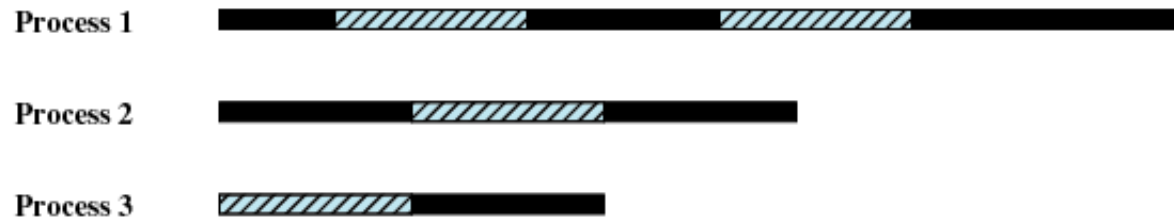
(b) Interleaving and overlapping (multiprocessing; two processors)
